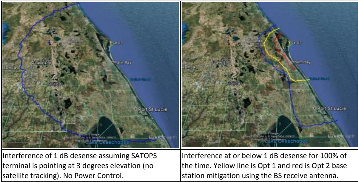
1667 Figure 4.2.5-6. 1 dB Desense for EVCF, baseline scenario showing impact of limiting SATOPS 1668 pointing direction, All Channel 1 Satellites.
