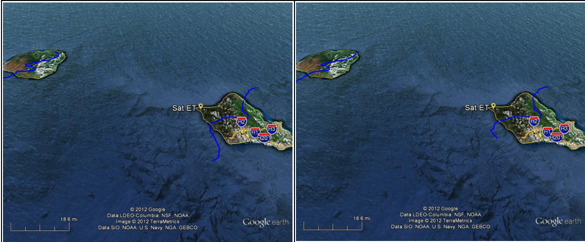
Interference of 1 dB desense assuming SATOPS terminal is pointing at 3 degrees elevation (no satellite tracking).
