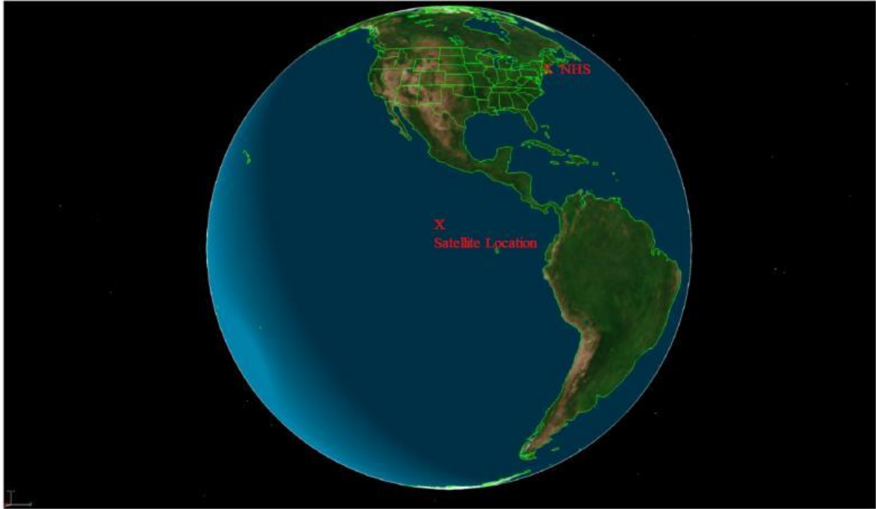
2022 Figure 4.2.6-4. Field of View of a Geostationary Satellite at 102 Degrees West Longitude.
