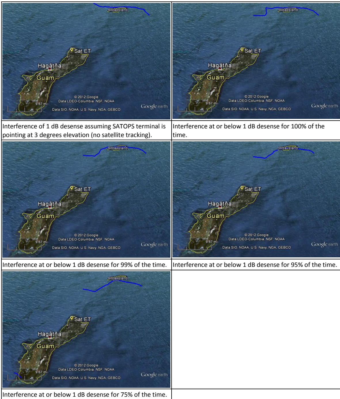
Figure 4.2.3-50. 1 dB Desense for GTS, baseline scenario at various percentages of time, Channel 2.
