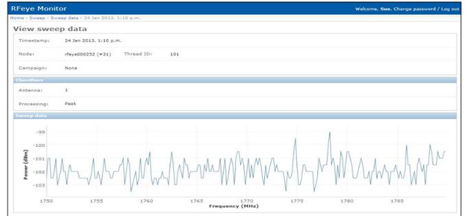
Both frequency and time domain spectral captures can be graphically displayed within the web interface, with controls for scale and range-zoom via simple click and drag. As with other data, the sweep and time data can be filtered by Node ID, campaign, date/time, antenna input and spectral processing, and also output to CSV.
