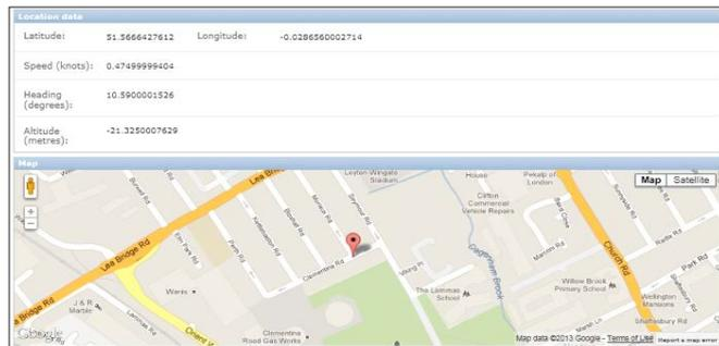
The location of each RFeye Node in the network can be viewed on a map within RFeye Monitor. Mobile RFeye Nodes will display their historical location according to the data timestamp selected. Full NMEA data along with Node management data including unit temperatures, supply voltages and currents, as well as disk usage statistics are all made available to enable comprehensive status management of the RFeye network.
