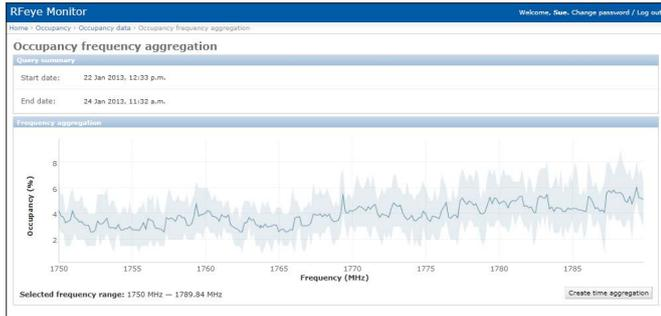
RFeye Monitor allows the user to run queries by individual Node or aggregated groups for occupancy by time or frequency during any selectable period of time. The Nodes take measurements at the requested rate based on power measured above a threshold, in accordance with ITU recommendation SM 1880 for occupancy.
