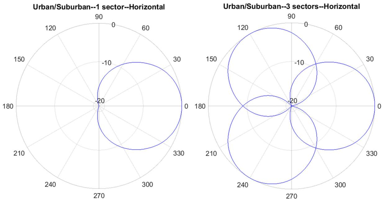
**Figure 3. Urban and Suburban Horizontal Antenna Gain Pattern**
