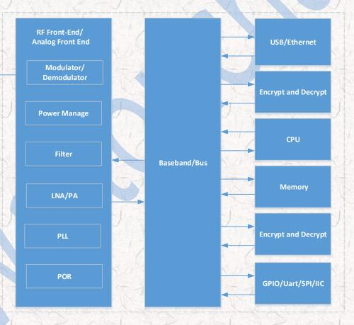
Figure 2.5: The project's tag IC solution block diagram
