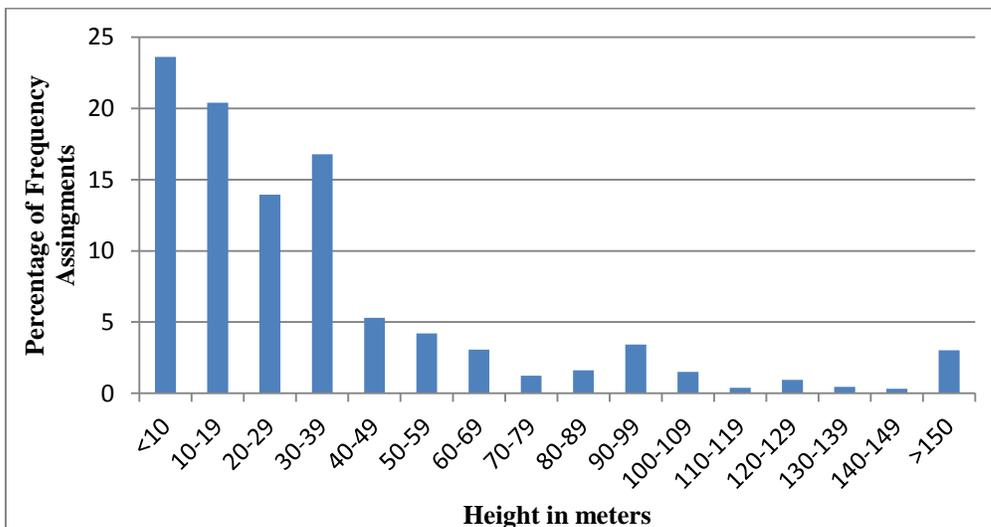
**Figure 3: Distribution of Fixed Station Antenna Height Above Ground Level in the 406.1 - 410 MHz Band**
