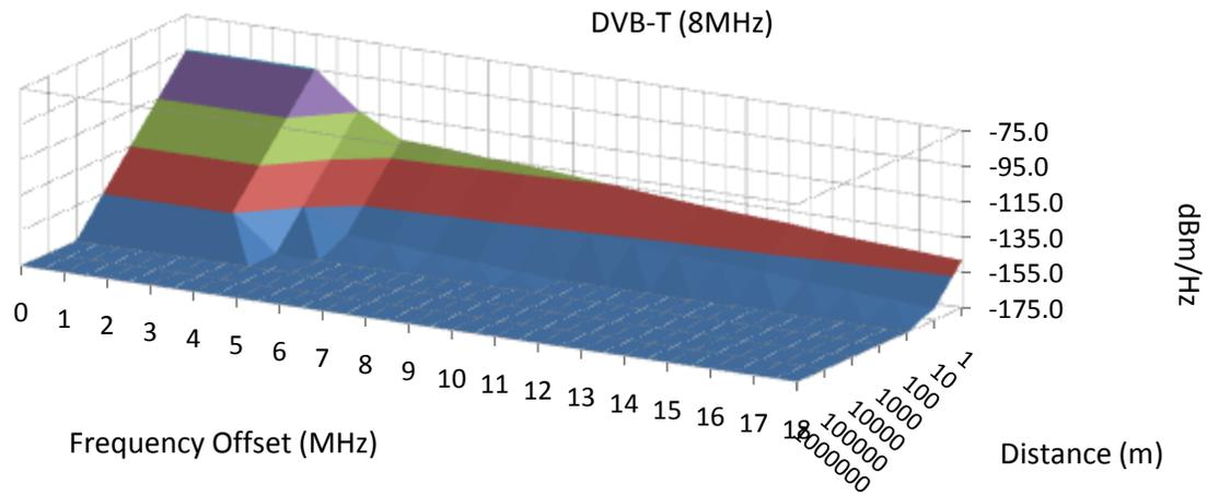
Figure 9 500 mW Transmitter attenuated by Building and at 20 meter Height
