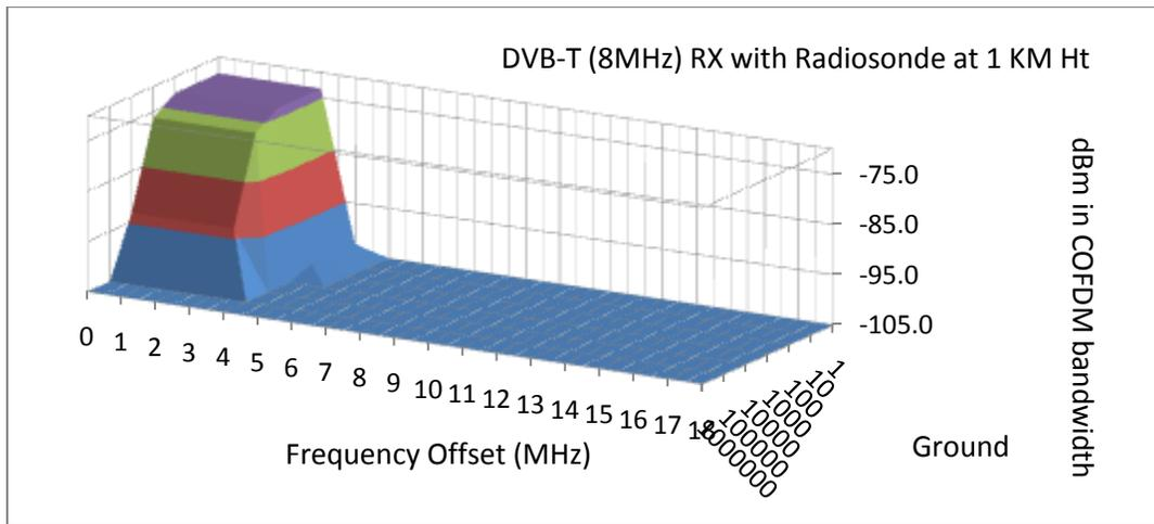
Figure 8 Estimate of Received Interference from Radiosondes vs. Frequency Offset vs. Distance Smooth Earth
