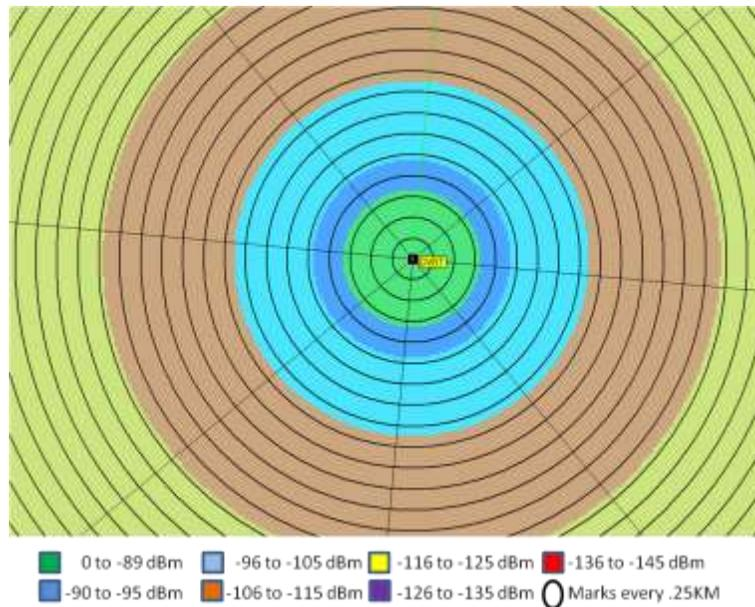
Figure 10 500 mW Transmitter at 2 meter Height on smooth earth in 8 MHz Bandwidth
