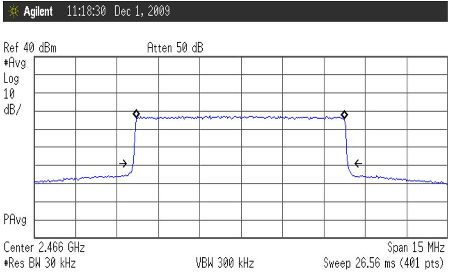
**Figure 6 COFDM 8 MHz transmitter Spectrum**
