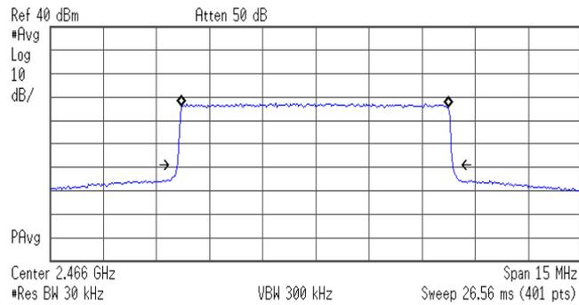
i Example of measured transmitter power spectral mask:
