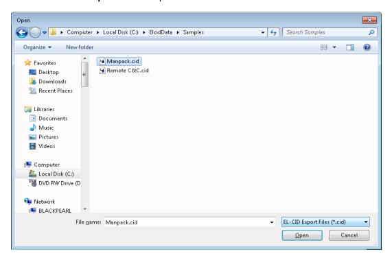
Select the **Manpack.cid** file and click **Open**. (The net effect here is to choose the Manpack.cid file, which is in the Samples folder within your El-CID data folder.)
