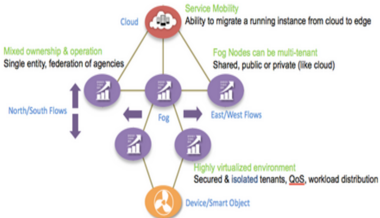
Figure 2. Fog Computing Nodes between Devices and Cloud from Cisco
