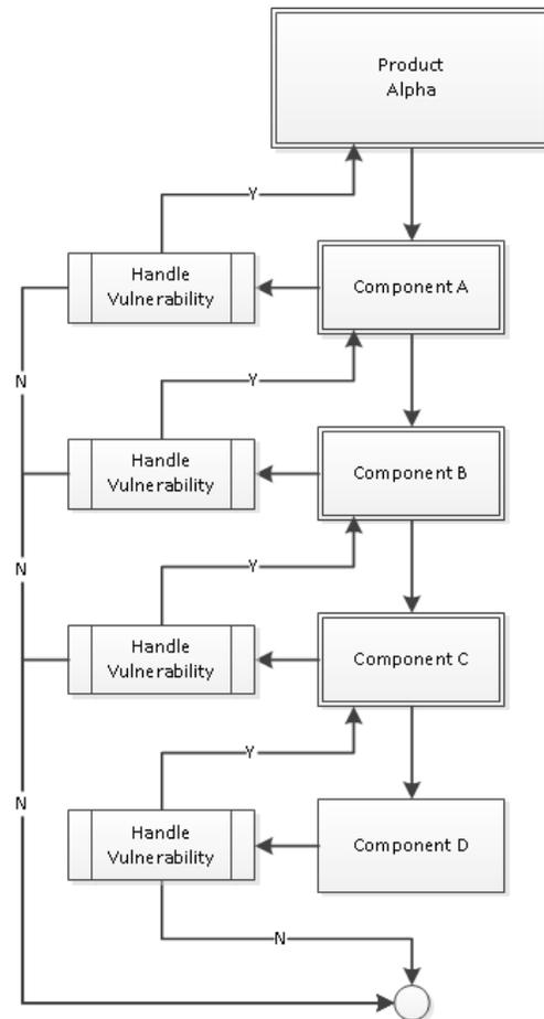
Figure 2: Vulnerability Mitigation Flow - depicting a vulnerability and mitigation flow back up to the product.
