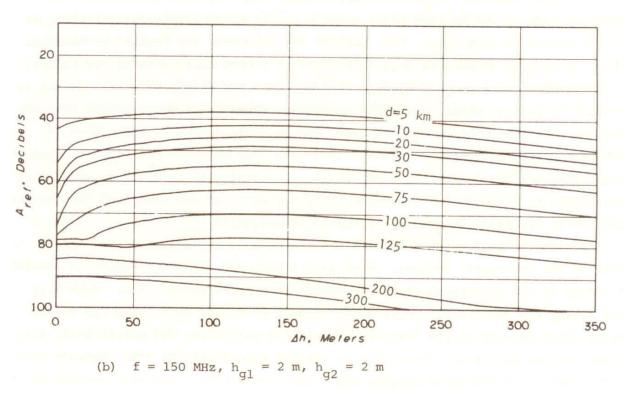
Figure 4. The reference attenuation versus  $\Delta h$  for selected distances.
