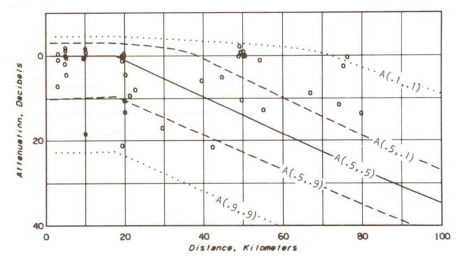
Figure 12. Predicted and observed values of attenuation versus distance for the R3 data. The predictions assumed the transmitters were sited very carefully.
