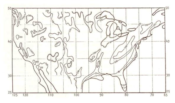
Figure 3. Contours of the terrain irregularity parameter  $\Delta h$  in meters. The derivation assumed random paths and homogeneous terrain in 50 km blocks. Allowances should be made for other conditions.
