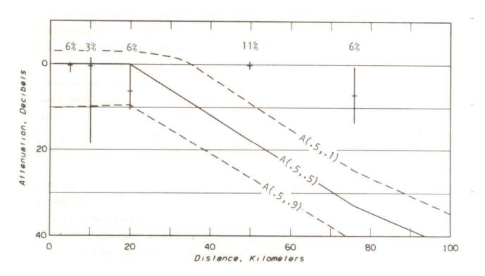
Figure 11. Predicted and observed medians for the R3 data. The bars indicate confidence levels for the sample medians at approximately 10% and 90%.
