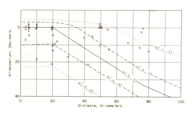
Figure 9. Predicted and observed values of attenuation for the R3 data. Assumed parameters: f=410 MHz,  $h_{g1}$ =275 m,  $h_{g2}$ =6.6 m,  $\Delta h$ =126 m,  $N_s$ =250 N-units.
