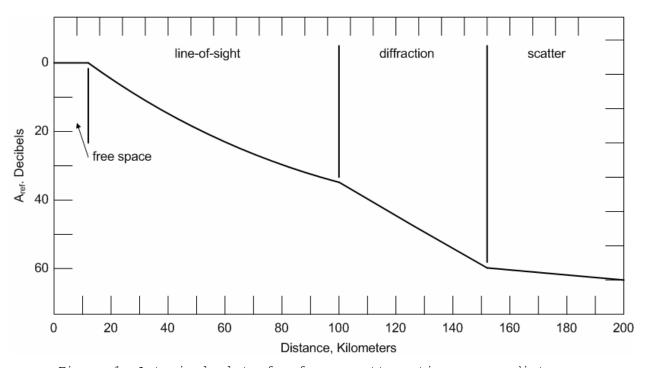
Figure 1. A typical plot of reference attenuation versus distance.
