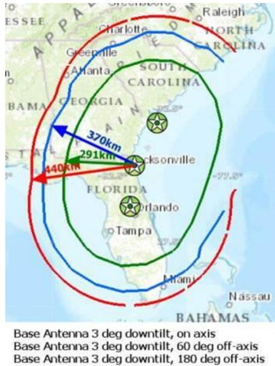
Figure 4-23. Navy TTNT to LTE Base Stations, NAS Jacksonville, FL
