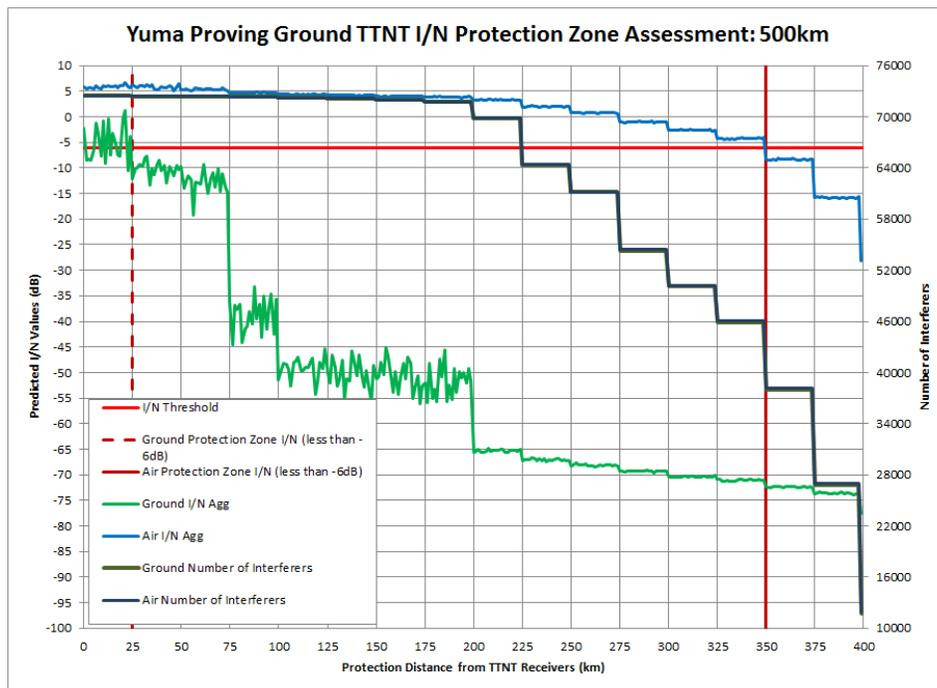
**Figure 4-22. UEs to Army/USMC TTNT, Yuma Proving Ground**
