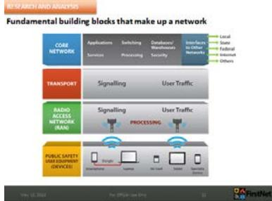
I know that some of you here today are technical and some are not so I wanted to step through a diagram of the components of an LTE network.
