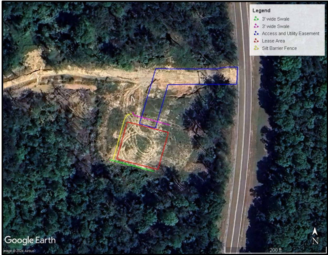
Figure 2. 2024 Google Aerial Image with Revised Project Area Details. Not to Exact Scale; for Illustrative Purposes.
