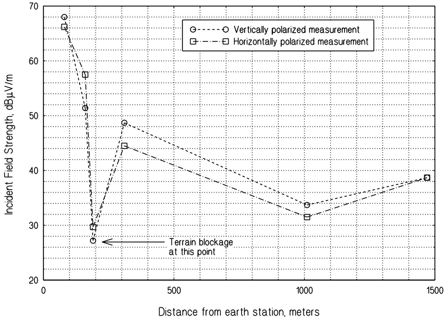
Figure 9. Incident field strength as a function of distance from the Mt. Jackson fixed satellite service (FSS) earth station.
