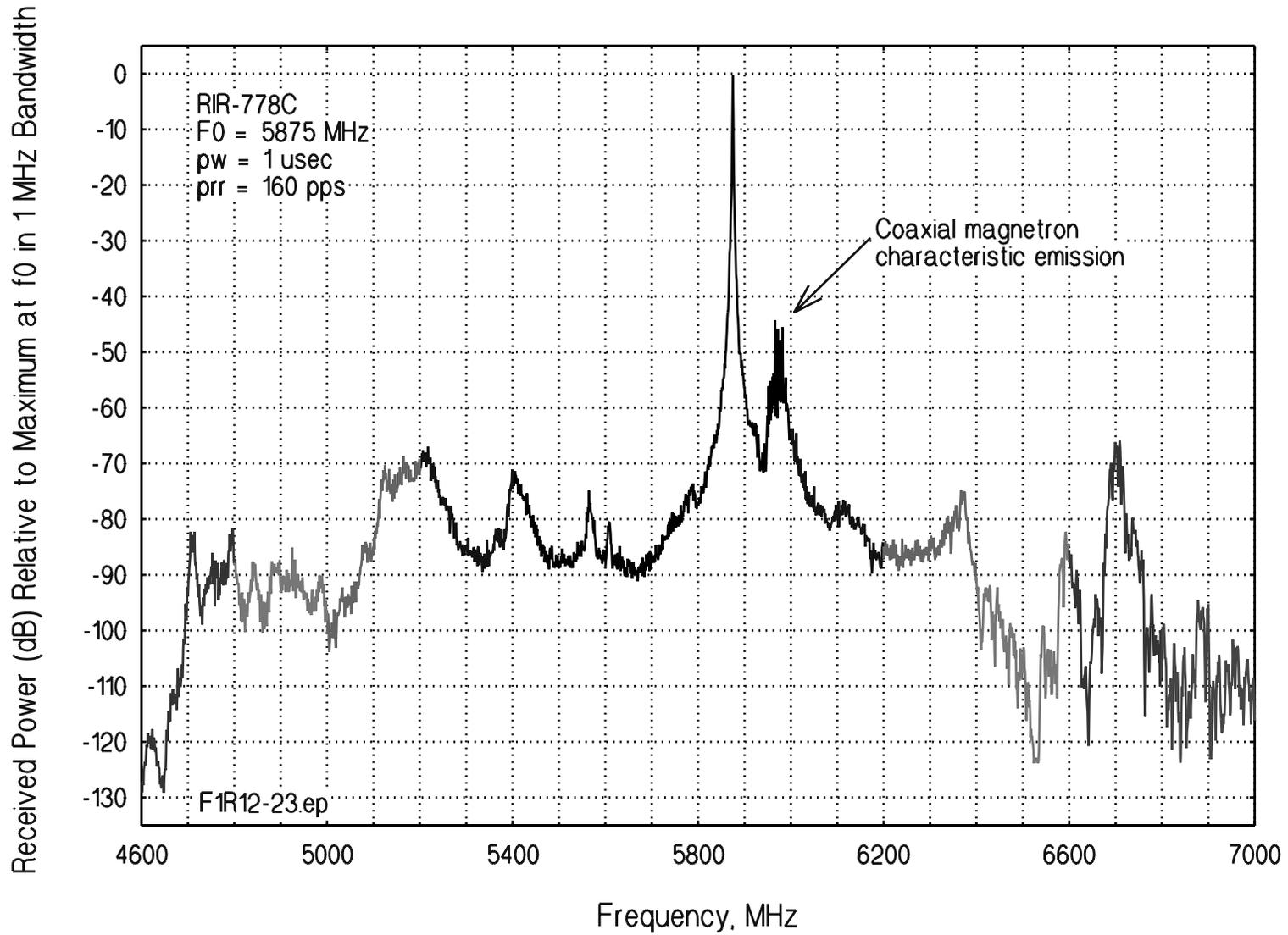
Figure 7. RIR-778C radar spectrum. Peak level at 5875 MHz is +163 dBuV/m at a distance of 3.0 km. This spectrum is typical of coaxial magnetron radars [9].
