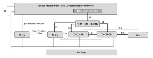
Figure 1: O-RAN architecture with 5G components
