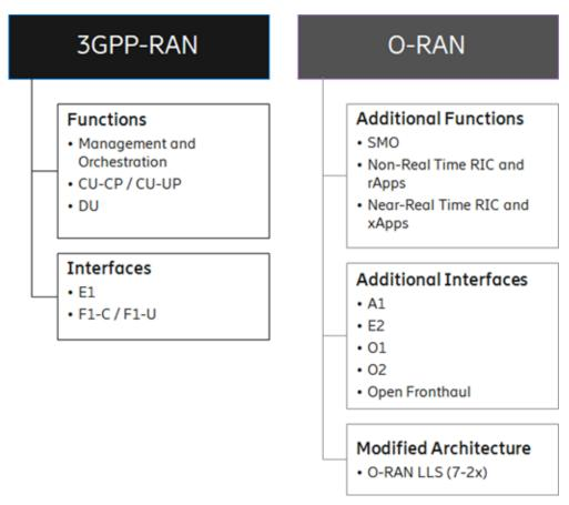
Figure 9: 3GPP and O-RAN functions and interfaces (source: Ericsson)
