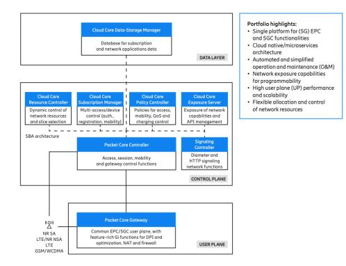
Figure 6: Dual-mode 5G Core
