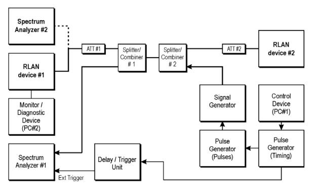
Figure B1: Conducted DFS Measurements - Test Set-Up
