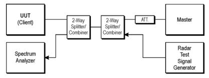
For the purposes of the test, the UUT as well as other unlicensed U-NII devices used in the set-up may be equipped with a specific user interface to allow monitoring of the behavior of the different devices of the set-up during the tests.
