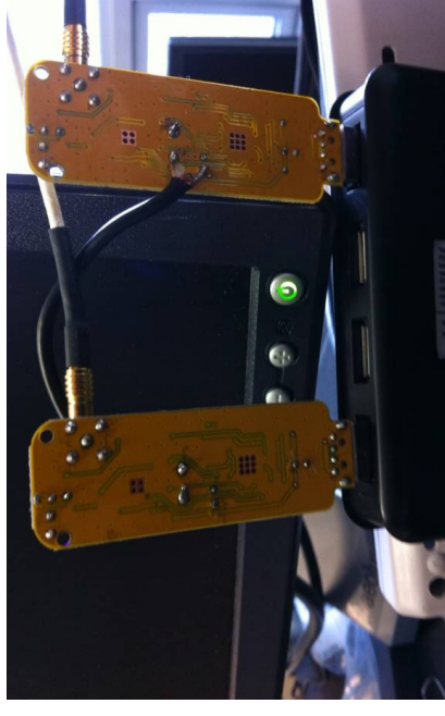
Hub with the right usb port orientation for rtl dongles
