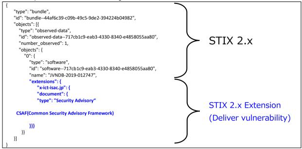
Figure 5: embedded CSAF in STIX
