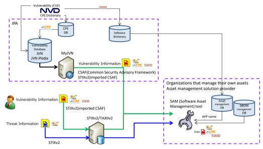
Figure 4: VDB, SBOM and STIX collaboration data flow
